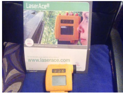
6. Trimble LaserAce 1000 Range finder with digital compass
